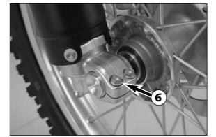
To install the front wheel, lift it into the fork, position and mount the axle shaft. Mount the collar nut **⑤**, tighten the clamping screws **⑥** on the right fork leg axle passage to prevent the axle shaft from turning and tighten the collar nut to 40 Nm (30ft.lb).
