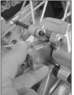
Insert the left brake pad into the brake caliper and secure it with the bolt. Insert the right brake pad and push the bolt [3] into the brake caliper up to the stop. Reattach clips [2].
