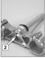
Remove the collar screw from the lower triple clamp and pull out the steering stem. Thoroughly clean all parts. Turn the steering stem 180° and insert it in the triple clamp. Apply Loctite 243 to the thread of the collar screw [2] and turn all the way in.
