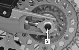
lar nut to 80 Nm, push the rear wheel forwards so that the chain tensioners
