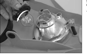
Slightly depress the bulb, turn it approx.  $30^\circ$  counterclockwise and pull it out of the socket.
