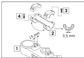
For this purpose, remove screws **[3]** of the handlebar clamps and screws **[4]** of the handlebar support. Position the handlebar support, and tighten screws **[4]** to 40 Nm (30 ft.lbs). Mount the handlebar and handlebar clamps, and tighten screws **[3]** to 20 Nm (15 ft.lbs). The gap between the handlebar support and the handlebar clamps should be the same size in the front and in the rear.
