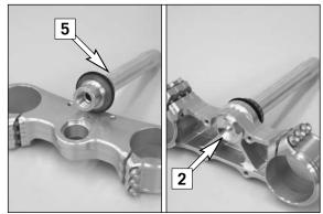
Remove the collar screw from the lower triple clamp and pull out the steering stem. Thoroughly clean all parts. Turn the steering stem 180° and insert it in the triple clamp. Apply Loctite 243 to the thread of the collar screw [2] and turn all the way in.
