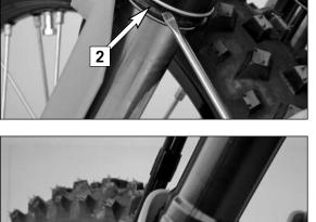
Clean the dust-protection bellows, outer tubes, and fork tubes thoroughly, and oil them thoroughly with Universal oil spray (Motorex Joker 440) or engine oil. Then, push the dust-protection bellows into the outer tubes by hand.
