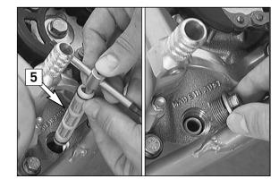
To mount the long oil screen [5], place it on an approx. 300 mm (12 in) long pin-type key or a similar tool. Insert the pin-type key through the opening into the bore of the opposite engine casing wall. Then, push the oil screen into the engine casing as far as possible. Remove the pin-type key, mount the plug and tighten it to 15 Nm.
