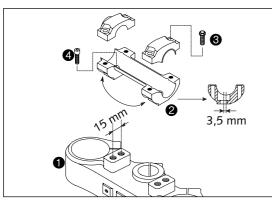
For this purpose, remove screws ③ of the handlebar clamps and screws ④ of the handlebar support. Position the handlebar support, and tighten screws ④ to 40 Nm (30 ft.lbs). Mount the handlebar and handlebar clamps, and tighten screws ⑤ to 20 Nm (15 ft.lbs). The gap between the handlebar support and the handlebar clamps should be the same size in the front and in the rear.
