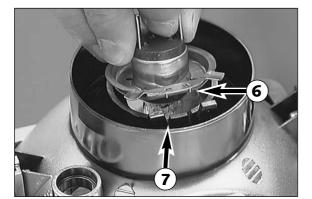
Insert a new lamp such that the noses ③ engage in the recesses ④. When doing so, do not touch the glass body of the lamp so that it remains free from fat. Engage retaining clip, mount rubber cap and connector. If the parking-light lamp is to be replaced, simply insert it in the holder. Reinsert parking-light lamp together with the holder.
