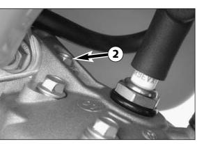
Remove screw **2** at the cylinder head. Reinstall it as soon as the cooling liquid emerges free of air bubbles (only for 125/200 engines).
