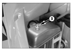
Remove the screw **③** on the right radiator.
