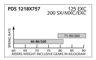
According to our experience, the damping rate of the compression stage can remain unchanged. The damping rate of the rebound stage can be reduced by a few clicks for a softer spring or increased by a few clicks for a harder spring.
