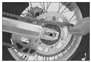
The rear wheel is remounted in the reverse order. Before tightening the collar nut to 80 Nm (60 ft.lb), push the rear wheel forwards so that the chain tensioners lie on the tension screws.
