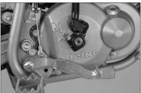
**Foot brake lever** The foot brake lever is located in front of the right footrest. The basic position can be adjusted to the seating position (see maintenance work).
