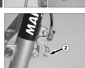
Mount the right brake shoe and fix with screw. Mount the left brake shoe and tighten the screw to 6 Nm. Mount the lock washer. Align brake shoes, mount front wheel (see chapter: Mounting the front wheel).
