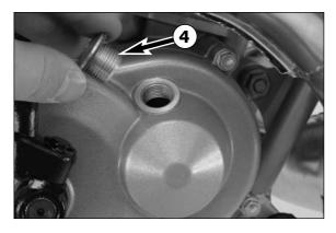
Remove stopper 4 and fill in 0.15 liters of automatic gear oil (Shell Donax TA). Mount the stopper and check the engine for tightness.
