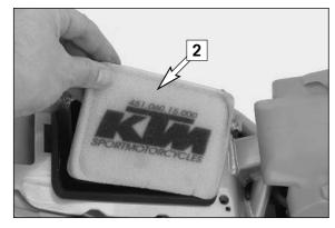
Thoroughly wash the foam filter in special cleaning fluid (Motorex Bio Dirt Remover) and allow it to dry well. Only press out the filter, do not wring it out under any circumstances. Oil the dry foam filter with a high-grade filter oil (Motorex Liquid Bio Power). Also clean the air filter box. Check carburetor collar for damage and that it is filled correctly.
