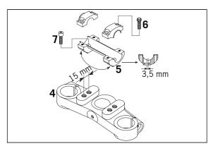
For this purpose, remove screws [6] of the handlebar clamps and screws [7] of the handlebar support. Position handlebar support, and tighten screws [7] to 40 Nm. Mount handlebar and handlebar clamps, and tighten screws [6] to 20 Nm. The gap between the handlebar support and handlebar clamps should be the same size in the front and in the rear.
