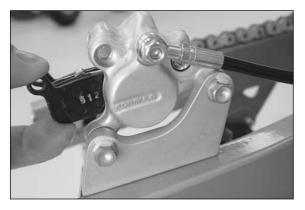
Slide new brake shoes into the brake caliper a fasten with the screw [5]. Tighten the screw to 10 Nm and mount the locking screw [4]. Mount the rear wheel and actuate the foot brake lever until you can feel the pressure point.
