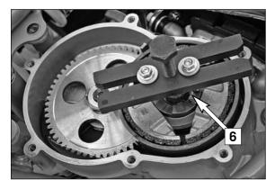
Screw the extractor (special tool item no. 590.29.021.044) onto the clutch hub **[6]** with the M5x50 screws, hold the extractor and remove the centrifugal clutch from the crankshaft by screwing in the extractor screw.
