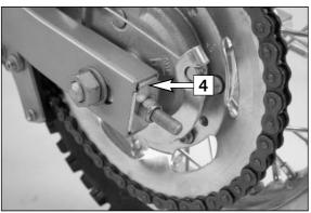
To mount the wheel reverse the procedure described above. Always hook the brake backing plate into the swing arm support. Before tightening the hexagon nut of the wheel spindle, ensure that the supporting plates [4] are resting against the swing arm. Additionally, check that the rear wheel is aligned with the front wheel. Tighten the hexagon nut to 40 Nm.
