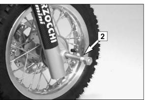
Jack the motorcycle up by the frame so that the front wheel is suspended above the ground.
