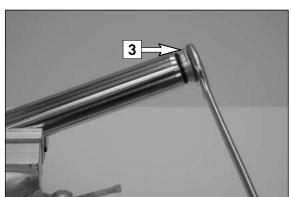
Clamp the fork leg into a vise (use protective jaws) and remove the plugs [3]. Take the preload spacer and the spring out of the fork tube. Remove screws [4] at the underside of the slider tubes and pull the fork tubes out of the slider tubes.
