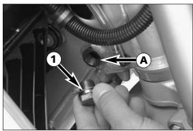
Fill 0.6 liters (0.16 US gallons) of engine oil into the can and remove the plug • next to the steering head. Introduce the plastic hose into the vent hole •, (see page 30) and fill 0.6 liters (0.16 US gallons) of engine oil into the frame's front tube. Remove plastic hose, start engine, and let it idle (approx. 20 seconds) until oil escapes at the hole •. As soon as oil begins to leak out, switch off the engine, mount the plug and gasket and tighten to 25 Nm.
