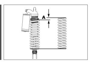
Loosen the locking ring **1** with the hook wrench from the tool set. Change the spring preload with the adjusting ring **2** and retighten the locking ring.
