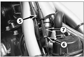
If a correction is necessary, start by removing the tank. Slide back the protection cover **⑤**. To set the backlash, loosen the counter nut **⑥** and turn the adjusting screw **⑦** accordingly. Then, fasten the counter nut and slide the protection cover back on.
