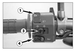
The indicator switch **3** returns to central position after actuation. Press flasher switch towards switch housing to switch off the flasher.
