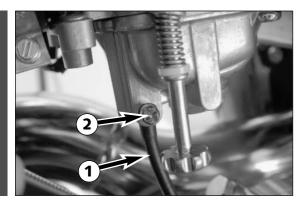
Open the drain plug  ${\bf 2}$  (turning it counterclockwise) by several turns, and drain the fuel from the float chamber.
