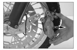
After mounting the front wheel, slide the brake caliper to the brake disc. Remove the grease from the threads of both screws 4 and apply Loctite 243. Tighten the screws with 40 Nm.
