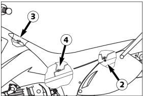
To mount the seat hook it into the oval head screw, lower the rear part of the seat and push the whole seat forwards. If necessary push the middle of the seat slightly down to let the retaining bracket ② engage with the seat. Finally fasten the seat with the corresponding screw.
