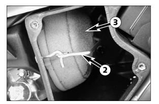
Mount the air filter on the filter holder, position in the filter box (make sure to center) and fix with the retaining clip. Check whether the air filter is positioned correctly and mount the filter box cover.
