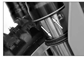
Clean dust-protection bellows, outer tubes, and fork tubes thoroughly, and oil them thoroughly with oil-spray (Motorex Joker 440) or engine oil. Then, push dust-protection bellows into the outer tubes by hand.
