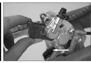
Press both brake shoes into the brake caliper and fix with bolt **[2]**. Mount the locks **[1]**. Tighten bolt **[2]** to 5 Nm (3,7 ft.lb).
