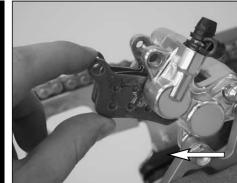
Press both brake shoes into the brake caliper and fix with bolt [2]. Mount the locks [1]. Tighten bolt [2] to 5 Nm (3,7 ft.lb).
