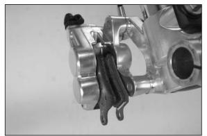
Mount the right brake shoe and fix with screw. Mount the left brake shoe and tighten the screw to 4 Nm. Mount the lock washer. Align brake shoes, mount front wheel (see chapter: Mounting the front wheel).
