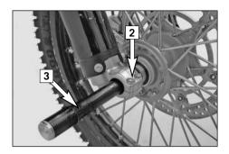
To install the front wheel, lift it into the fork, position and mount the axle shaft [3]. Mount the collar nut [1], tighten the clamping screws [2] on the right fork leg axle passage to prevent the axle shaft from turning and tighten the collar nut to 40 Nm (30ft.lb).
