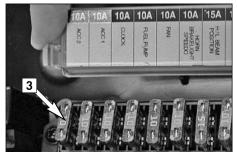
Fuses ACC 1 and ACC 2 [3] are designed for accessories with a maximum power consumption of 10 amperes each. Fuse ACC 2 also protects the carburetor heaters from short circuits.
