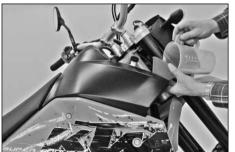
Completely fill the radiator with cooling liquid. Mount the radiator cap and move the motorcycle into a horizontal position again. Fill the compensating tank with cooling liquid until it reaches a level between the MIN and MAX mark. Close the compensating tank.
