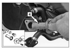
Carefully pull the oil screen [4] out of the oil tank.
