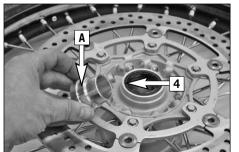
Before remounting the front wheel, clean and grease the shaft seal rings [4] and the bearing surface [A] of the distance bushings and mount the distance bushings. Slightly push back the brake pads with a screwdriver. Set up the front wheel facing in the running direction.
