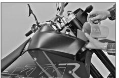
Completely fill the radiator with cooling liquid. Mount the radiator cap and move the motorcycle into a horizontal position again. Fill the compensating tank with cooling liquid until it reaches a level between the MIN and MAX mark. Close the compensating tank.
