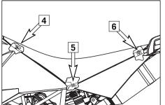
To mount the seat, attach the seat to the oval head screw [4], lower the seat in the back while sliding it towards the front. Both noses [5] should fit into the frame. Insert the catch bolts [6] in the lock housing and push the seat down in the back until you hear the catch bolts snap into place.
