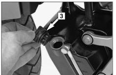
Unscrew the plug [3]. Add 2.5 liters (0.7 USgal) of fully synthetic engine oil according to the JASO MA Norm (e.g. Motorex Power Synt 4T) and remount the plug. Start the engine and allow to run warm in neutral until 4 bars on the temperature indicator light up. Switch off the engine and check the engine oil level (see Checking the engine oil level).
