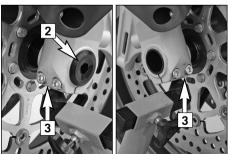
Loosen the collar screw [2] and the clamping screws [3] on both fork leg axle passages. Unscrew the collar screw approx 8 turns, press on the collar screw with your hand to push the wheel spindle out of the fork leg axle passage and remove the collar screw. Hold the front wheel while you pull out the wheel spindle.
