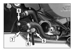
Remove the drain plug [5] from the oil tank and allow the oil to drain into a vessel. Remove the screws [6] and tilt the connector [7] to the side.
