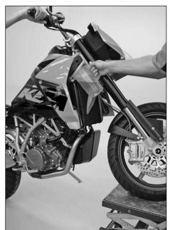
Add cooling liquid until it runs out of the vent holes without bubbles and immediately mount the screw to prevent air from entering the radiator.
