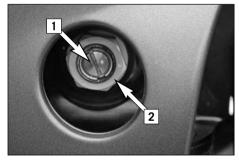
The adjusting screw [1] for the low-speed range can be adjusted with a screwdriver.
