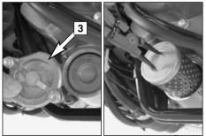
Place the motorcycle on a level surface. Remove the 4 screws, take off the underride protection and place a receptacle for the used oil under the engine. Remove the oil drain plug [1], take off the cap [2] and pull the oil sieve out of the engine case with a pair of pliers.
