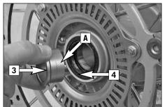
Before remounting the front wheel, clean and grease the shaft seal rings [4] and the bearing surface [A] of the distance bushings and mount the distance bushings (wide distance bushing in the left shaft seal ring). Slightly push back the brake pads with a screwdriver. Set up the front wheel facing in the running direction (see arrow [B] on the tire).
