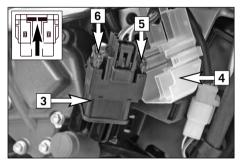
Lift the starter relay [3] out of the bracket, remove the cap [4] and check the main fuse [5]. A spare fuse [6] (30 ampere) is also plugged into the starter relay.
