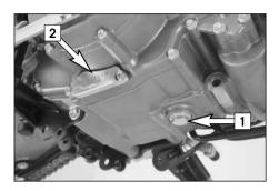
Changing the engine oil and the oil filter, cleaning the oil screen
