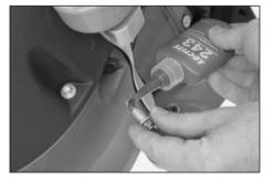
Apply Loctite 243 to the thread of the 4 screws, mount the underride protection and tighten the screws to  $25\ \text{Nm}$ .
