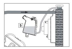
A mixture of 50% antifreeze and 50% distilled water is used as the cooling liquid. How ever, the anti-freeze protection must be at least -25° C (-13° F). Aside from antifreezing protection, this mixture also provides great corrosion protection which is why it must not be replaced by pure water.
