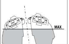
The 990 Adventure has 2 tanks with 1 filler cap each. Both filler caps can be locked and are equipped with a tank vent system. To open, insert the ignition key, turn  $45^{\circ}$  in a clockwise direction and fold up the filler cap. The ignition key can be pulled out to open the other filler cap. Simply press on the filler cap to close.
