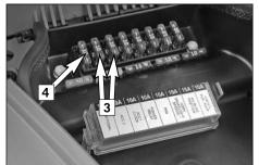
The ACC 1 / CLOCK and ACC 2 fuses [3] are designed for accessory equipment with a maximum current consumption of 10 amperes each. The respective connectors for this equipment are provided under the headlight cover. For more information, contact an authorized KTM workshop.
