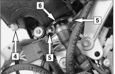
Remove the drain plug [4] on the oil tank and allow the oil to drain into a receptacle. Remove the screws [5] and tilt the oil return valve [6] to the side.
