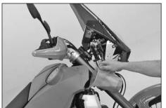
To be able to completely bleed the cooling system, raise the motorcycle approx. 50 cm in the front.
