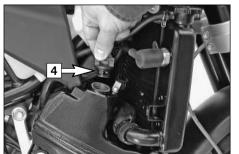
Unscrew the plug [4] and refill engine oil. Wait 20 seconds and check the oil level again. The quantity of oil between the MIN and MAX marks is 0.3 liter. Mount the plug and check the engine for leaks.
