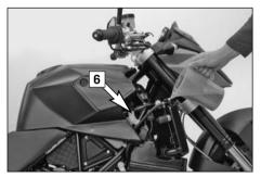
To completely bleed the cooling system, the motorcycle must be raised approx. 50 cm (20 in) in the front.
