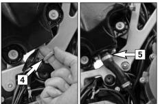
Mount the oil drain plug on the oil tank with a new seal ring and tighten to 20 Nm.
