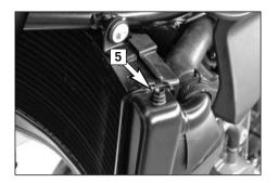
Remove the bleeder screw [5] on the left side of the radiator.
