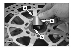
Before you remount the front wheel, clean and grease the shaft seal rings [5] and the bearing surface [A] of the distance bushings and mount the distance bushings (wide distance bushing in the left shaft seal ring). When mounting the distance bushing, be careful not to press the sealing lips towards the inside. position the front wheel according to the running direction shown by the arrows [B] on the rim.
