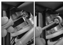
The adjusting screw [2] for the low-speed range can be adjusted with a screwdriver.
