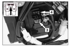
Pull the connector [1] out of the bracket, remove the cap [2] and check the main fuse [3]. A spare fuse [4] (30 amperes) is also plugged into the bracket.
