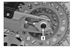
The rear wheel is remounted in the reverse order. Before tightening the collar nut to 80 Nm, push the rear wheel forwards so that the chain tensioners lie on the tension screws.
