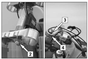
Loosen the clamp screws and take the fork legs out of the triple clamps. Loosen the collar screw [2] on the lower triple clamp 2 turns.
