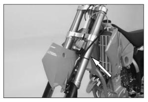
To adjust the offset, dismount the front wheel and remove the front wheel fender.
