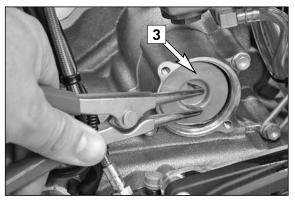
NOTE: The 250 SX-F engine only has one oil filter insert [3].
