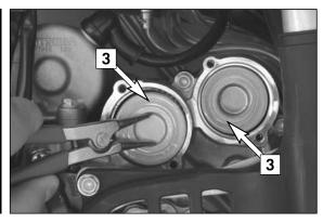
Using circlip pliers, pull the oil-filter inserts [3] out of the housing. Clean the oil filter cover, the sealing surfaces of the O-rings and the engine casing. Check the O-rings of the oil filter covers for damage and, if necessary, replace them.
