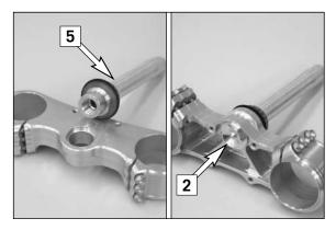
Remove the collar screw from the lower triple clamp and pull out the steering stem. Thoroughly clean all parts. Turn the steering stem  $180^{\circ}$  and insert it in the triple clamp, tighten the collar screw all the way to the stop.
