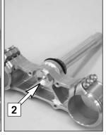
Remove the collar screw from the lower triple clamp and pull out the steering stem. Thoroughly clean all parts. Turn the steering stem  $180^{\circ}$  and insert it in the triple clamp, tighten the collar screw all the way to the stop.
