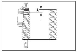
ADJUSTMENT VALUES – SPRING PRELOAD [A] STANDARD PRELOAD . . . 5 mm (0.20 in)
