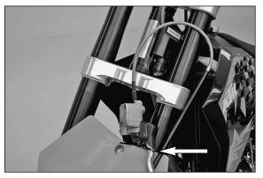
To adjust the offset, dismount the front wheel and remove the front wheel fender.
