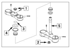
The offset is set to 20 mm in the condition at delivery.
