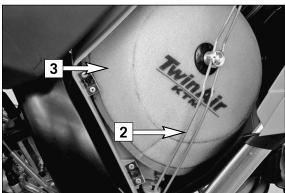
Thoroughly wash the air filter in special cleaning fluid (Motorex Twin Air Dirt Bio Remover) and allow it to dry well. Only press out the filter, do not wring it out under any circumstances. Oil the dry air filter with a high-grade filter oil (Motorex Twin Air Liquid Bio Power). Also clean the air filter box. Check the carburetor collar for damage and that it is filled correctly.
