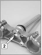
Remove the collar screw from the lower triple clamp and pull out the steering stem. Thoroughly clean all parts. Turn the steering stem  $180^{\circ}$  and insert it in the triple clamp. Apply Loctite 243 to the thread of the collar screw [2] and turn all the way in.
