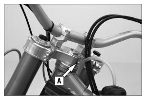
Mount the lower triple clamp, upper steering head bearing, protection ring, O-ring, upper triple clamp and the blind screw.
