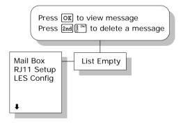
The **Mailbox** feature handles messages being sent from the LES operator. If a call is made to a terminal, which is busy, switched off, etc. the LES operator may offer the facility to record a short message. When the terminal again becomes operational a message is sent indicating that the LES operator has recorded a short message for the terminal.
