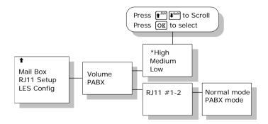
2-wire phones, connected to the RJ11 interfaces, may vary in sensitivity. The output volume from the interfaces can therefore be adjusted. The volume can be set to **High**,
