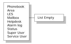
The **Mailbox** feature is not supported by all LES operators. The feature handles messages sent from the LES operator. If a call is made to a terminal, which is busy, switched off, etc. the LES operator may offer the facility to record a short message. When the terminal again becomes operational a message is sent indicating that the LES operator has recorded a short message for the terminal.
