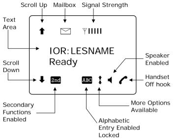
The display contains a set of symbols, which together with the 4 indicators situated below the display gives continuous indication of current status.
