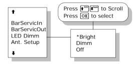
The brightness of the 4 Handset LED's can be adjusted. To change the brightness level, select the **LED Dimm** menu and adjust the value with **1**<sup>Edf</sup> and **1**<sup>Cond</sup>. Setting can be adjusted to Bright, Dimm and Off. Default value is Bright.
