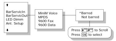
All outgoing calls on a specific service can be barred. Scroll through the services with  $\mathbf{E}^{\text{Eff}}$ . Select the service with  $\mathbf{O}\mathbf{K}$ . The service can then be set to 'Barred' or 'Not barred' with  $\mathbf{E}^{\text{Eff}}$ .
