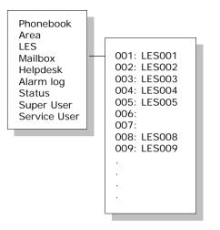
The **LES** list contains a list of those LES operators, which may be selected as gateway to the terrestrial network. The last used LES will be marked with \* and this LES will also be the first LES tried next time the terminal is logged on. Use OK to select. The Area selected in section 4.3.2 A, will decide, which LES's will be available for selection (see section 4.4.23 LES Config for further information about LES configuration).
