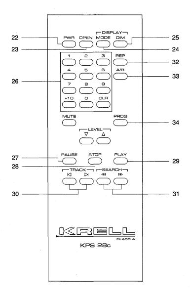
**Compact Disc Compact Disc Special Play Functions Transport Functions Functions** 32 Rep (Repeat) Key 22 Pwr (Power Key) 26 Direct Track Access 33 A/B Key 23 Open Key Keypad 34 Prog (Program) Key **Compact Disc** 27 Pause Key **Display Functions** 28 Stop Key 24 Display Mode Key 29 Play Key 25 Display Dim Key 30 Track Forward and Back Keys
