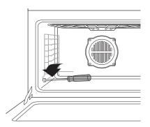
Take hold of the oven door on both sides and close it slowly. When the oven door is about half-closed, the hinges will fall out of the catches.
