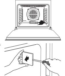
Carefully lever out the glass cover with a screwdriver.
