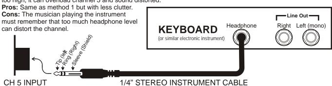
Method 3: Mono using mono Line out -
