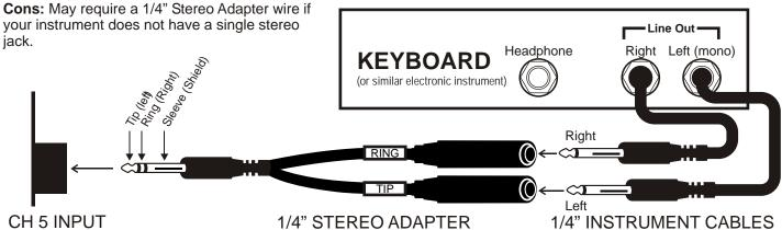
Method 2: Stereo using Headphone output-
