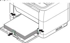
**Note** Load an amount of paper that fits under (does not contact) the tabs on the width guides.
