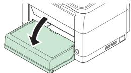
**Note** When storing the cassette, or when using paper larger than A4/Letter, remove the cassette cover.
