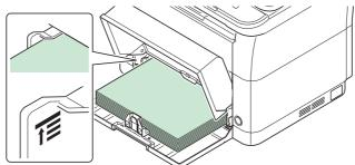
When using A6 paper, load the paper as shown in the illustration.
