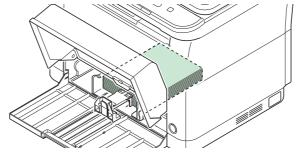
When loading an envelope, load as shown in the illustration.
