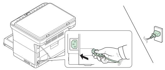
2 Connect the other end of the power cord to a power outlet.
