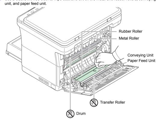
2 Use a clean, lint-free cloth to wipe dust and dirt off the metal and rubber rollers, conveying
