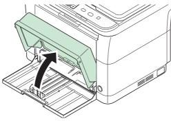
**Note** When using paper that is larger than A4/Letter, remove the cassette cover. Gently press on both the left and right sides of the cassette cover and pull.
