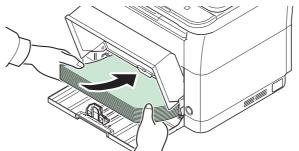
**IMPORTANT** Adjust so that there is no gap between the paper length guide and the paper.
