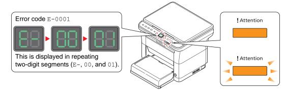
**Note** If the indicators light or flash repeatedly in manners not described above, a service error has probably occurred. Switch off the power switch, unplug the power cord, and then plug the power cord back in and switch on the power switch. This may clear the error. Even if the error is not cleared, contact your service representative.
