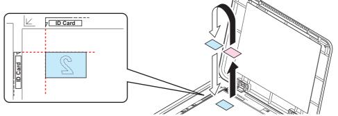
7 Press [Start]. The front and back sides of the card are copied on one sheet of paper.
