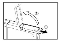
2 Insert the battery pack (BP-780S) supplied with the camera.
