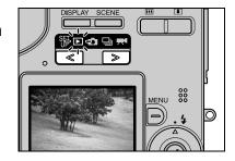
2 Press ▶ on the 4-way button to scan forward through the photographed images. Press ◀ to scan backward through the images.
