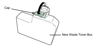
Insert the new waste toner box as shown in the figure below. When the box is set correctly, it will snap into place.
