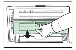
Open the fuser cover and remove the jammed paper by pulling it out.
