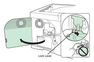
**NOTE:** Remove the waste toner box as gently as possible so as not to scatter the toner inside. Do not let the opening of the waste toner box face downward.
