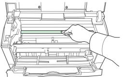
Insert the developer unit together with the toner container, back into the machine.
