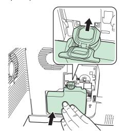
6 Make sure that the waste toner box is correctly inserted and close the left cover.
