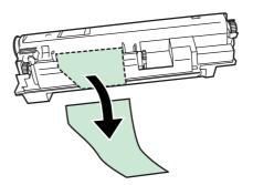
7 Set the new toner container in the printer and push down on the top of the toner container to install it firmly in place as shown in the figure below.
