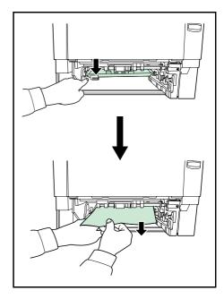
Insert the paper cassette into the slot in the printer. The printer warms up and resumes printing.
