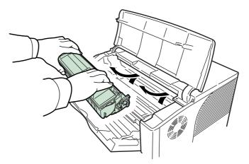
3 Use a lint free cloth to clean dust and dirt away from the metal Registration Roller (metal).
