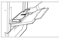
Remove the jammed paper on the multi-purpose tray up and towards the right.
