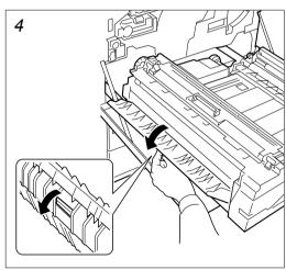
Open the fuser access cover by pressing the green-colored lock lever.
