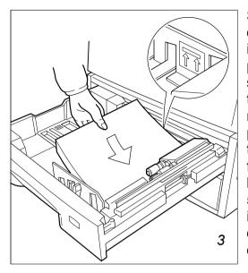
Square the edges of the paper and insert into the paper feed cassette. Be sure that the paper does not exceed the paper limit indicators. The paper feed cassette can hold up to about 500 sheets. Printing is performed on the underside of the paper.
