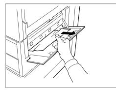
Open the paper feeder side cover according to the number in place of #, top (1) to bottom (3). Pull the paper outward. Close the side cover.
