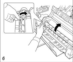
Raise the subcover by grasping the clip marked as *A* on the rear side while removing the paper.
