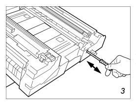
Gently pull the green cleaning knob out and push it back in. Repeat this 5 to 7 times. This cleans the separation charger inside.
