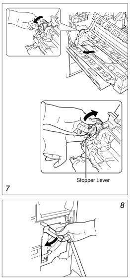
If the paper is pinched between the rollers, turn the wheel as shown towards you.
