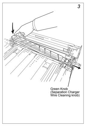
Hold the new separation charger unit so that the projecting pin is in front of you and pass the green knob (separation charger wire cleaning knob) through the secondary transfer unit Press the back side to lock the unit
