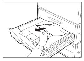
Open the paper cassette according to the number in place of #, top (1) to bottom (6). Remove the paper in the paper cassette.
