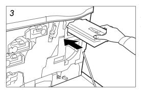
Insert the new toner container all the way in. The container is locked automatically when it is properly seated.
