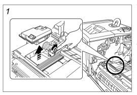
Tilt to the right the lever on the righthand side of the bottle and remove the bottle. Do not place the removed bottle upside down.
