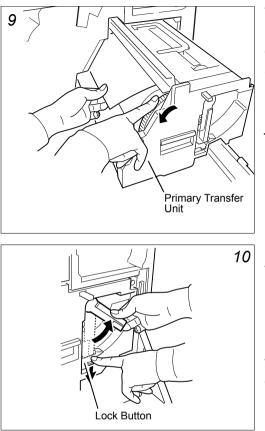
Turn the wheel (with gear teeth) on the right-hand side of the primary transfer unit. Remove the jammed paper.
