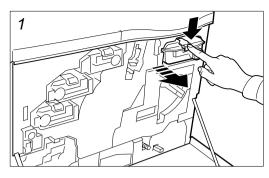
While pressing down the bluecolored lever at the end of the toner container, pull the toner container out.
