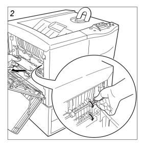
Remove the jammed paper. If the paper does not go easily, refer to section [Paper Jam — Paper Feed Unit] on page 17.
