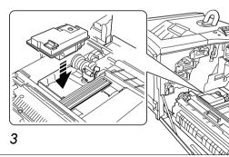
The old waste toner bottle has a cap. Remove the cap (black) on the top of the bottle and put the cap onto the opening. This is to prevent the toner from spilling.
