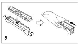
Put the old oil unit in the cover and put it in the plastic bag (contained in the oil unit kit) and discard it.
