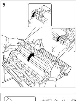
Open the fuser top cover by simultaneously pulling the two lock levers.
