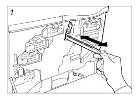
Cleaning the main charger wire — Grasp the tab of the cleaning knob (green) and gently pull out and push it back in 3 to 5 times.
