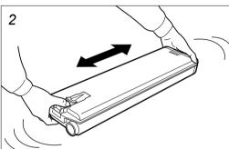
Take the new toner container out of the toner kit. Hold the container and shake the container back and forth at least 5 times.
