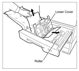
Open the duplexer drawer. Open the plastic covers and remove paper under the covers and rollers.
