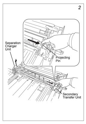
Remove the old separation charger unit from the secondary transfer unit. When you pull the projecting pin on the front end of the separation charger unit towards you as shown, the back end of the separation charger unit lifts up. Hold the back end of the separation charger unit to remove it.
