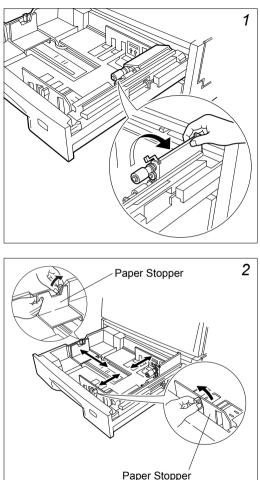
Pull out the paper feed cassette until it stops. Lift the paper feed roller located on the right side of the cassette upright.
