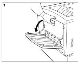
Open the face-up tray. Open the side cover by pulling the handle.
