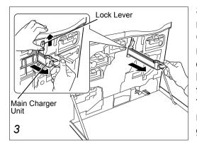
Slightly lift the main charger unit. Gently pull the main charger unit out and push it back in. Repeat this 2 to 3 times. These movements clean the grid at the bottom.
