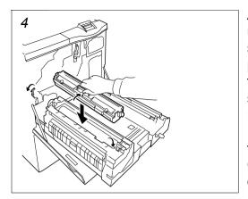
Attach the new oil unit. Seat it securely by pressing on the front and rear sides (the **PUSH HERE** areas). Push the paper feed unit back in. Close the front cover.
