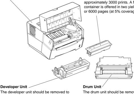
The developer unit should be removed to allow for cleaning tasks every time the toner container is replaced.
