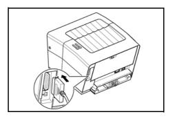
**NOTE:** Use a parallel printer cable that complies with IEEE 1284 standards. For optimum performance, install the printer close to the computer. The connection cable should be shielded and no longer than 3 meters (10 feet) long.
