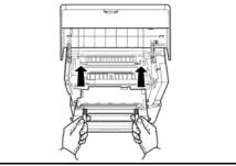
6 Insert the *Developer Unit* together with the *Toner Container*, back into the machine.
