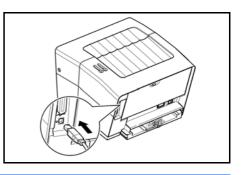
**NOTE:** Use a USB cable with a rectangular Type A plug and a square Type B plug. The USB cable should be shielded and no longer than 5 meters (16 feet) long.
