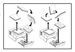
**NOTE:** Nothing will be printed on the instruction sheet. If the paper is curled, straighten it out before loading the paper in the cassette.
