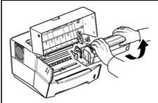
3 Using the green handles lift the Drum Unit out of the machine.
