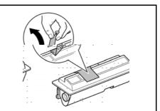
5 Install the new *Toner Container* in the printer. Push firmly on the top of the container at the positions marked PUSH HERE, until you hear a click.
