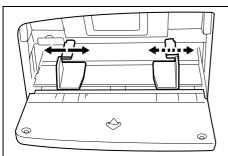
**2** Adjust the paper width guides to the width of the envelope.
