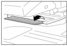
When stapling 11  $\times$  17", 8 1/2  $\times$  14", A3 or B4 paper, open the finisher tray extension to ensure that the paper does not fall out of the tray.
