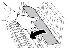
Remove the jammed paper.If you cannot remove the paper, proceed with the next step.
