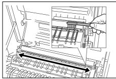
**15** Run the brush from side to side along the separator as shown to remove any soiling.
