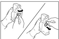
**3** Peel the sticker off the waste toner box and remove the cap.
