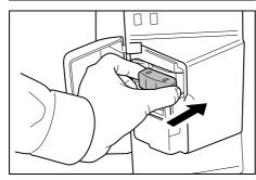
Reinsert the staple holder into the slot of the staple unit. The staple holder clicks locked when fully inserted.
