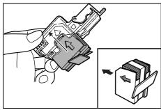
**4** Holding the staple holder in your left hand, insert a new staple case with your right hand in the direction of the arrow.
