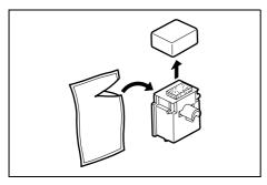
**8** Take the grid cleaner provided out of its bag and remove the cap.
