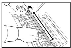
**16** Run the brush from side to side along the transfer roller as shown, rotating by the gear at the end, to remove any soiling.
