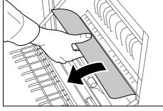
**3** Lift up the duplex unit and remove the jammed paper.
