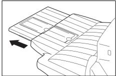
Adjust the ejected paper guide extension to the size of the paper.
