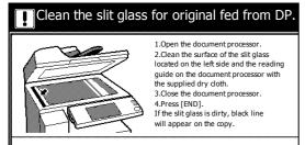
If black streaks or other soiling appears in copies when the optional document processor is used, clean the slit glass and white guide with the cleaning cloth provided. The message: Clean the slit glass for original fed from DP (Clean the slit glass for original fed) may be displayed if the slit glass requires cleaning. After cleaning, press [End].
