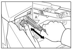
10 While gently holding the grid cleaner in place with your left hand, pull the main charger out fully and then push it back to a position where the roller **A** does not quite reach the white pad on the grid cleaner. Repeat 2 or 3 times.
