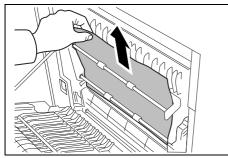
Lift up the duplex unit and remove the jammed paper.
