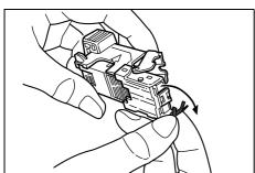
Remove the jammed staple from the end of the cartridge (staple-loaded side).
