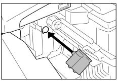
9 Align the grid cleaner with the notch and attach it to the machine.
