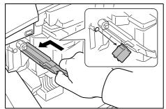
11 With the main charger pulled out about 5 cm (2 inches), remove the grid cleaner. Then push the main charger back in fully, applying pressure in the direction shown by the arrow so that the main charger is in its designated position.
