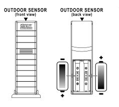
The Outdoor Temperature Sensor uses 2 x "AA", **Alkaline** batteries. To install and replace the batteries, please follow the steps below:
