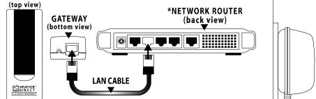
\*Your network router may look different than the diagram. Locate an available port on your router and plug in the included LAN cable. If you do not have a router, please visit www.weatherdirect.com/router
