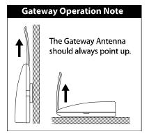
The Gateway should be installed indoors in an easy-to-reach location. Registration requires that you press the gray button on the Gateway. It can be mounted securely to the wall with the included mounting plate and drywall anchors.
