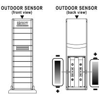
The Outdoor Temperature Sensor uses 2 x "AA", **Alkaline** batteries. To install and replace the batteries, please follow the steps below:
