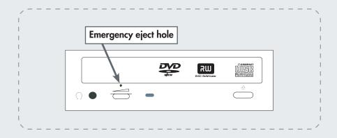
**CAUTION:** Make sure the LaCie Dupli Disc DVD121's power is off and the power cable is unplugged before attempting the emergency ejection procedure.
