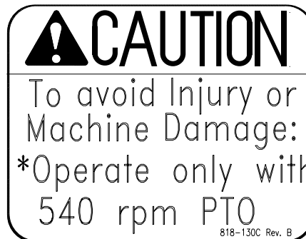
818-130C Caution! Use 540 rpm PTO only 818-240C Caution! Use 1000 rpm PTO only
