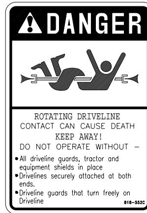
818-552C Danger: Rotating Driveline
