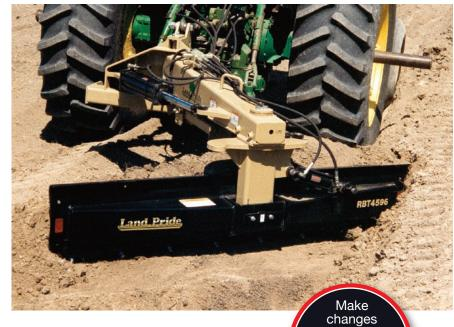
superior strength and resistance to bending or damage across the entire face of the moldboard. The lower edge of the tapered box beam is welded to the lower lip of the mold board. This makes the whole lower working edge of the moldboard into a 9/16" thick "super strong" formed and laminated mounting surface for the cutting blade.
