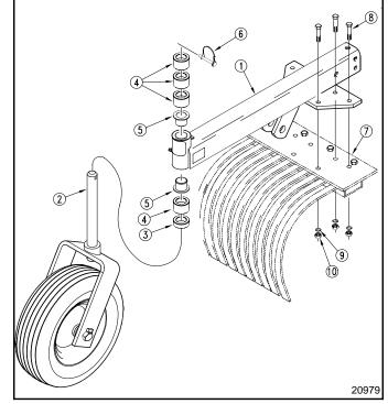
Gauge Wheel Assembly Right-Hand Assembly Shown Figure 2-3
