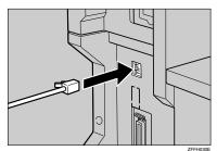
5 Connect the other end of the network cable to the network.6 Turn on the main power switch.
