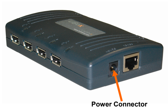
Figure 3-2. UBox Power Supply
