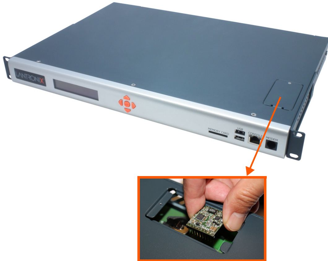
Figure 2-9 Internal Modem Location
