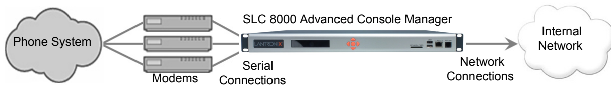
Figure 10-2 Remote Access Server
