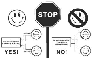
Two 4-ohm speakers, wired in stereo, will present a 4-ohm load to each channel of the amplifier. Most two-channel amplifiers will work well in this configuration.
