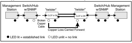
Loss of link at the fiber port is not propagated, as shown in the example below.
