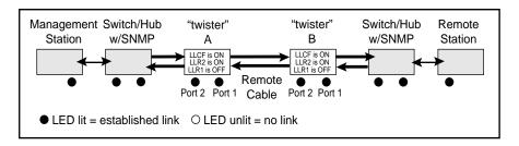
Example: If one of the optical conductors breaks (as shown in the diagram box below), "twister" B, with LLR2 enabled, will return a no-link condition to its link partner, "twister" A. On the fiber-to-fiber models with LLCF also enabled on both units, the no-link condition is carried forward to the switch/hub where a trap is generated to the management station. The network administrator can then determine the source of the loss.
