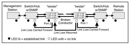
**IMPORTANT:** LLR must not be active on both ends of a configuration. If it is, the link can never be established.
