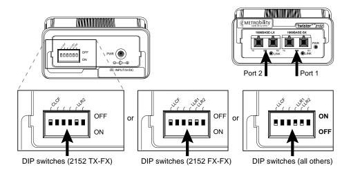
**NOTE:** The ON/OFF positions are not the same on all units. By default, all DIP switches are disabled.
