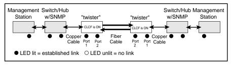
If a copper connection breaks, the "twister" will carry that link loss forward.
