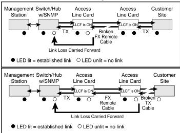
Important: When connecting a line card with LLCF enabled to an autonegotiating device, force both sides of the configuration to 100Mbps and either full or half duplex. This allows the card to immediately see link pulses and start passing data.
