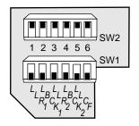
When setting DIP switches\*, the UP position is when the lever of the switch is pushed away from the circuit board. The DOWN position is when the lever of the switch is pushed toward the circuit board.
