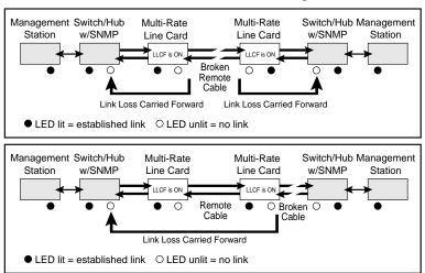
**NOTE:** Loopback takes precedence over LLCF. If LLCF and loopback are both enabled, LLCF functionality will be ignored for the port that is in loopback. LLCF will remain in effect for the port that is not in loopback.
