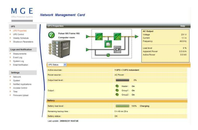
These measurements are available for AC to DC converter, Battery, DC to AC converter and automatic bypass. The measurements available in these boxes depend on the UPS range.
