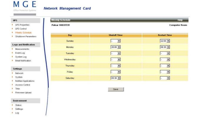
UPS configuration may prevent the shutdown and restart commands from being properly run. Read the UPS user manual for more information.
