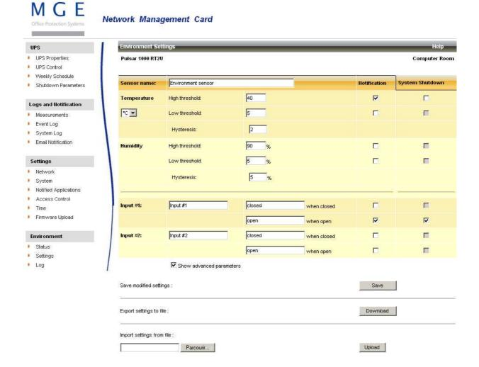
The environment sensor measures temperature, humidity and gives the status of the 2 contacts (used for door, alarms or generator unit).
