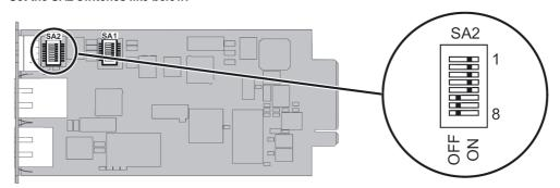
Set the SA1 switches to select the four wires configuration with no termination:
