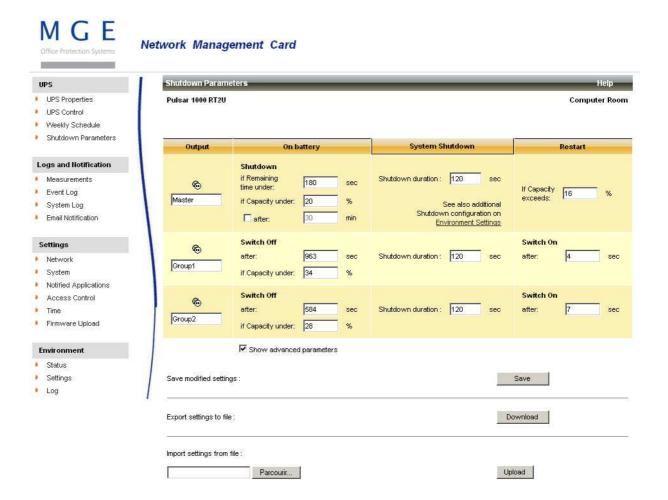
When you tick the Show advanced parameters option, extra parameters are displayed. These parameters enable, in particular, adjustment of certain thresholds related to the percentage of remaining battery charge level.
