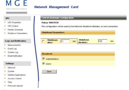
This page is used to define either the "shutdown" or the "notification" settings used by the Network Shutdown Modules that connect to Network Management Card. These settings are used by the Network Shutdown Modules if they are in central-configuration mode or if their configuration is not valid.
