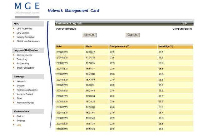
The two environment sensor measurements: Temperature and Humidity are recorded at an interval defined by the Environment log interval in the <a href="System settings">System settings</a> page.
