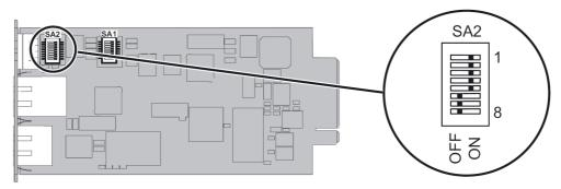
Set the SA1 switches to select the two wires configuration with no termination:
