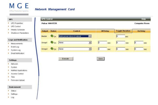
This page enables triggering of startup and shutdown sequences for the UPS main output and controlled outlets.
