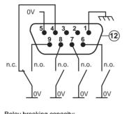
Relay breaking capacity: Vmax = 25V DC Imax = 10mA **n.o.**: normally open,
