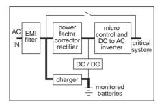
BYPASS MODE which is a default mode in the event of an inverter failure or overload in which the critical load is supplied AC through EMI/RFI filter:
