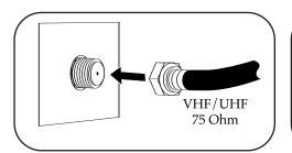
Connect the 75 ohm cable from the combination VHF/UHF antenna to the antenna jack.
