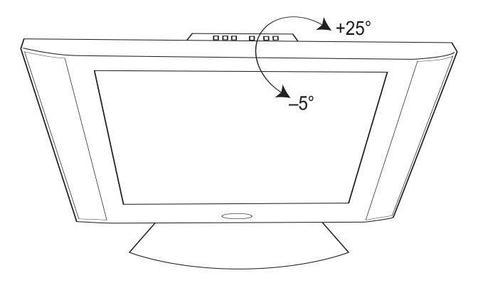
**NOTE:** Do not force the LCD monitor over its maximum viewing angle settings as stated above. Attempting this will result in damage to the monitor and stand.
