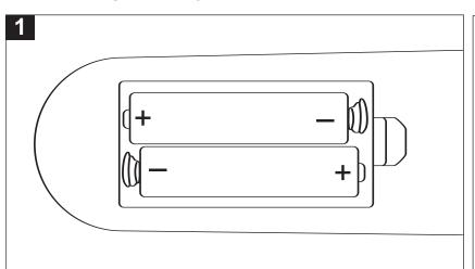
To remove the battery compartment cover, press in on the tab and then lifting it up.
