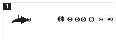
For private listening, insert an earphone into the EARPHONE jack on the rear of the unit. The speakers will be disconnected when the plug is inserted.
