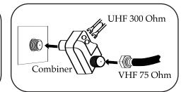
Connect the 75 ohm cable from the VHF antenna and the UHF antenna twin-lead wire to a combiner (NOT SUPPLIED). Attach the combiner to the antenna jack. **NOTE:** If your VHF antenna has a twin-
