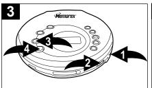
Adjust the VOLUME control ● and DBBS switch ❷ as desired. To **skip** forward or backward through the tracks on the disc, press the SKIP/SEARCH |◀◀ ❸ or ▶▶ button ④. To **search** forward or backward through the tracks on the disc, press and hold the SKIP/SEARCH |◀◀ ❸ or ▶▶ button ④.
