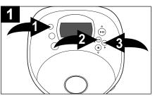
To repeat a single track, press the MODE button ● once; the Repeat 1 indicator will appear in the display. Press the Skip/Search (I◄◄)/◀ ❷ or (▶◄)/▶ ❸ button to select the specific track that you wish to repeat.
