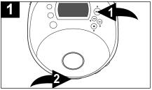
Press the Play/Pause (►II) /Power On/▲ button **①** to turn the unit on.
