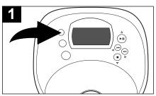
To repeat all the tracks on the CD, press the MODE button twice; the Repeat ALL indicator will appear in the display.
