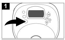
While in the Stop mode, press the PROG/ENTER button. The track number will blink and "P-01" will appear in the display.
