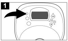
While in the Stop mode, press the MODE button three times (four times if an MP3 CD with multiple directories is inserted); "INTRO" will blink in the display.
