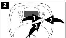
Select the first letter of a file you would like to listen to using the Skip/Search (I◄)/◀ ① and/or (I►)/► ② buttons. Press the Stop (I) /Power Off/▼ button ③ to access the lower letters.
