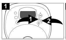
After you insert the disc into the CD player and the total number of tracks appear on the display, you may press either the Skip/Search  $(I \triangleleft \blacktriangleleft)/\blacktriangleleft \bigcirc$  or  $(\triangleright \bowtie)/\triangleright \bigcirc$  button to select a specific track for playback.
