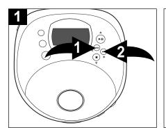
During playback, depress and hold either the Skip/Search (I◄◄)/◄ ◑ or (I►)/► ❷ button to move the player forward or backward within a track to locate a specific musical passage. The player will move forward or backward at high speed as long as the buttons are depressed. When you release the Skip/Search (I◄◄)/◄ ◑ or (I►)/► ❷ button, normal playback will resume.
