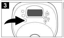
Press the PROG/ENTER button to memorize the track. Repeat steps 2 and 3 to program additional tracks up to a maximum of 24 tracks.
