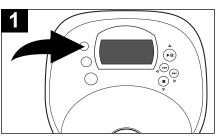
While in the Stop mode, press the MODE button four times (five times if an MP3 CD with multiple directories is inserted); "RAND" will blink in the display.
