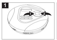
During playback, depress and hold either the Skip/TUNING IM or IM button to move the player forward or backward within a track to locate a specific musical passage. The player will move forward or backward at high speed as long as the buttons are depressed. When you release the Skip/TUNING IM or IM button, normal playback will resume.
