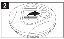
During playback, press and release the Skip/TUNING ₩ button once to move the player back to the beginning of the currently playing track. Press the Skip/TUNING ₩ button repeatedly to move the player back to lower-numbered tracks.
